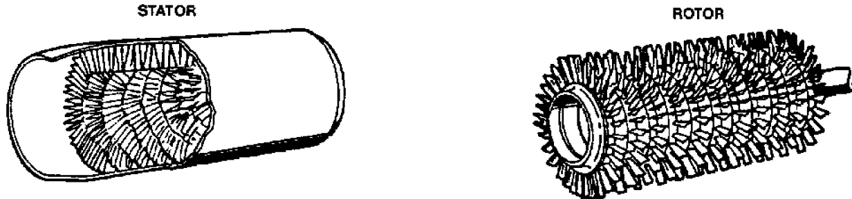
Figure 234-1-2. Rotor and Stator (Cutaway View) of Multistage Axial Compressor
